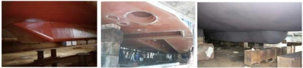
Figure 124: different installations for gondolas and blisters - sensors are located into a streamlined body outside the hull
